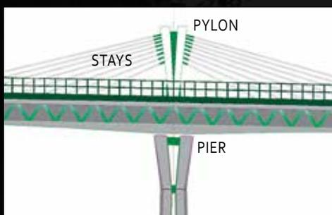
Basic parts of the cable-stayed bridge
