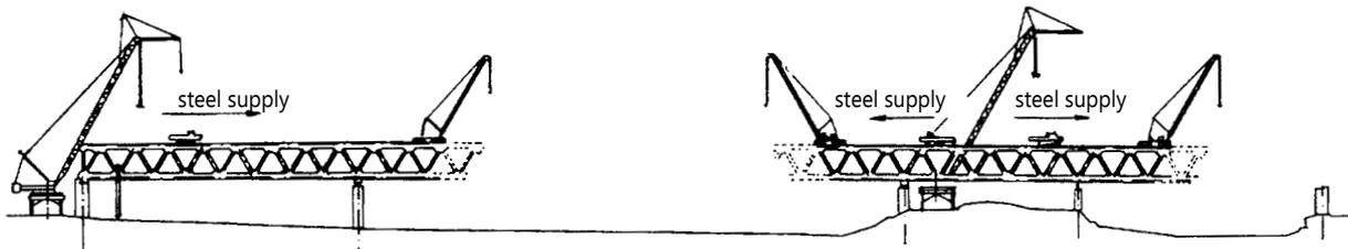
Steel truss bridge – cantilever erection method
