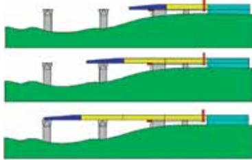
During the launching process, there are slide bearings placed on each pier on which the structure moves. In the case of a concrete bridge built by incremental launching technology, use is made of a so called steel launching nose placed at the front of the
