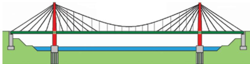
Hybrid structural system: combination of the suspension and the cable-stayed system
