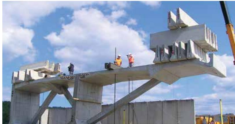
Experimental segment during the loading test
