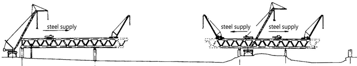
Steel truss bridge – cantilever erection method
