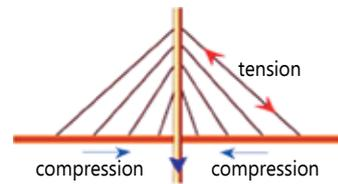
The basic structural behaviour of cable-stayed bridges may be best described by the diagram, where it can be seen that, for example, the pylon and the deck are subjected mainly to compression and the stay cables to tension forces (the pylon and the deck are at the same time subjected to bending moment).
